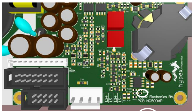
Figure 1 Placement of the bypass resistors
